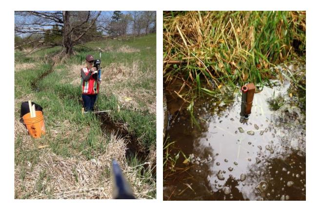
Visual flow monitoring and surface water level gauges installed by hand; no drilling required
