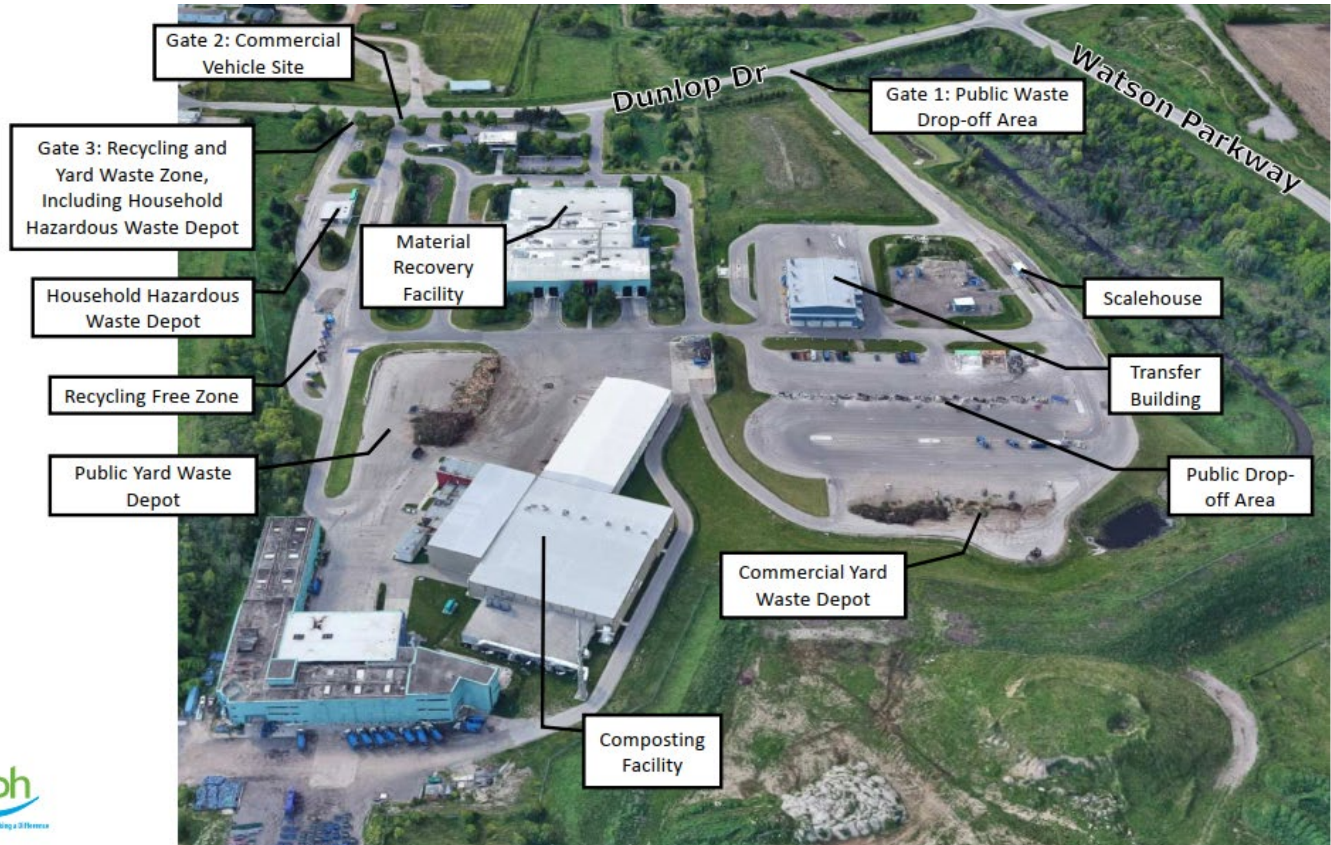
Figure 3: Waste Resource Innovation Centre Site Layout
