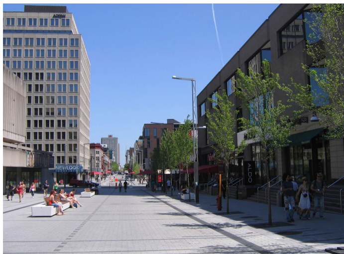
Curbless streets slow vehicles and allow pedestrians to seamlessly cross the road
